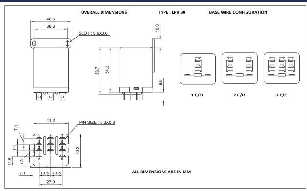
NOTE:-1) In case no tolerance shown in outline dimensions: Outline dimension 1mm, tolerance should be ±0.2mm
